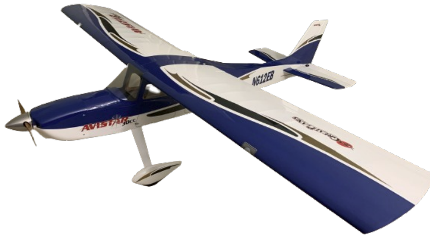
Figure 4: The as-purchased, used Great Planes Avistar 30cc in a taildragger (conventional landing gear) configuration, without flaps, and with an electric propulsion system.
