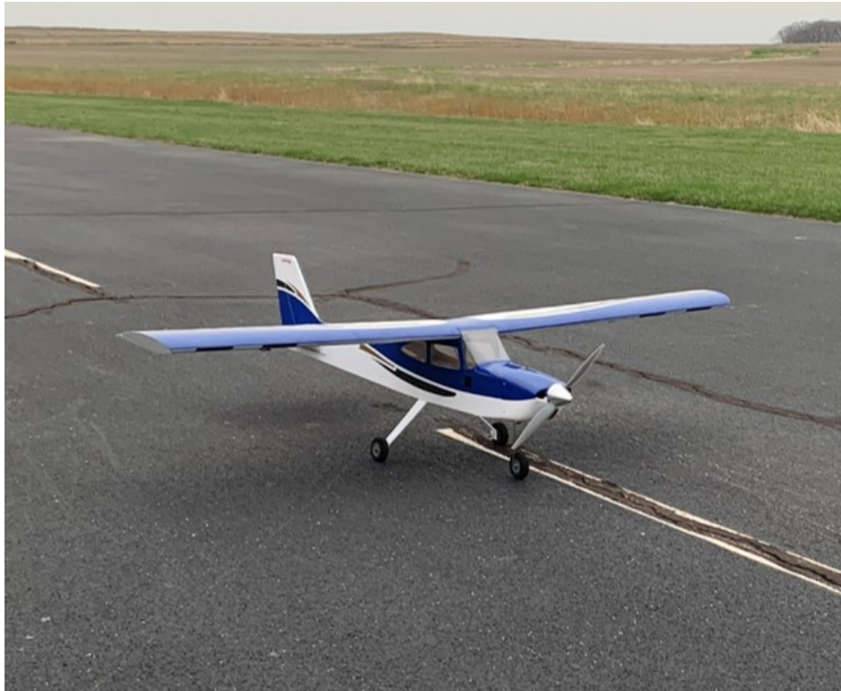
Figure 1: The flight-ready, 90.5 in (2.3 m) wingspan Great Planes Avistar 30cc.
