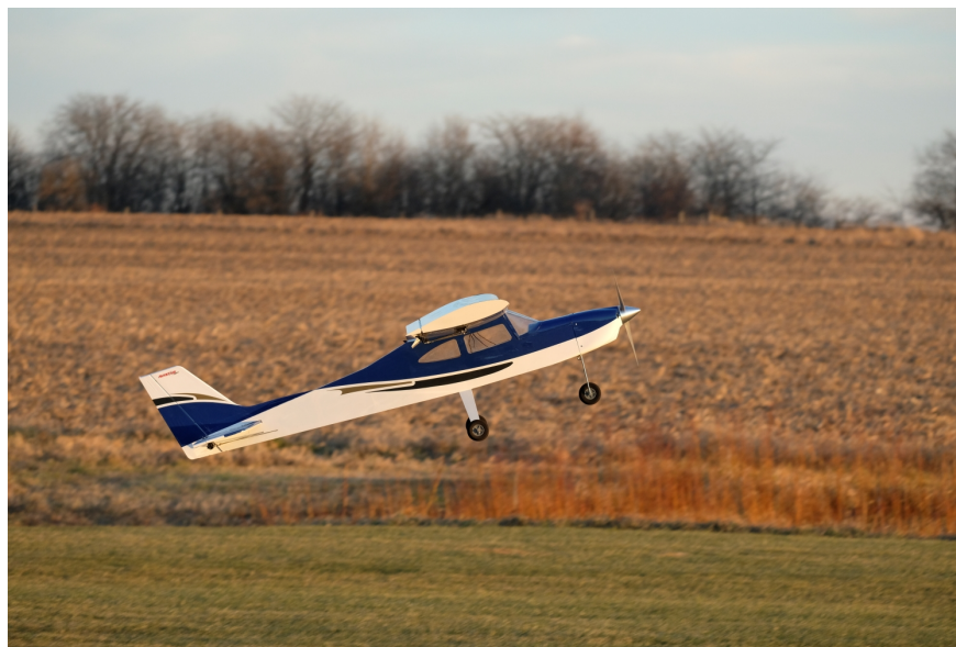
Figure 6: The un-instrumented Avistar 30cc being flown with full-flaps at slow speeds with a high angle-of-attack.
