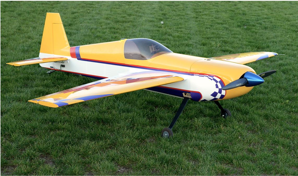
Figure 1. A photograph of the 35%-scale Extra 260 UIUC AeroTestbed aircraft.
