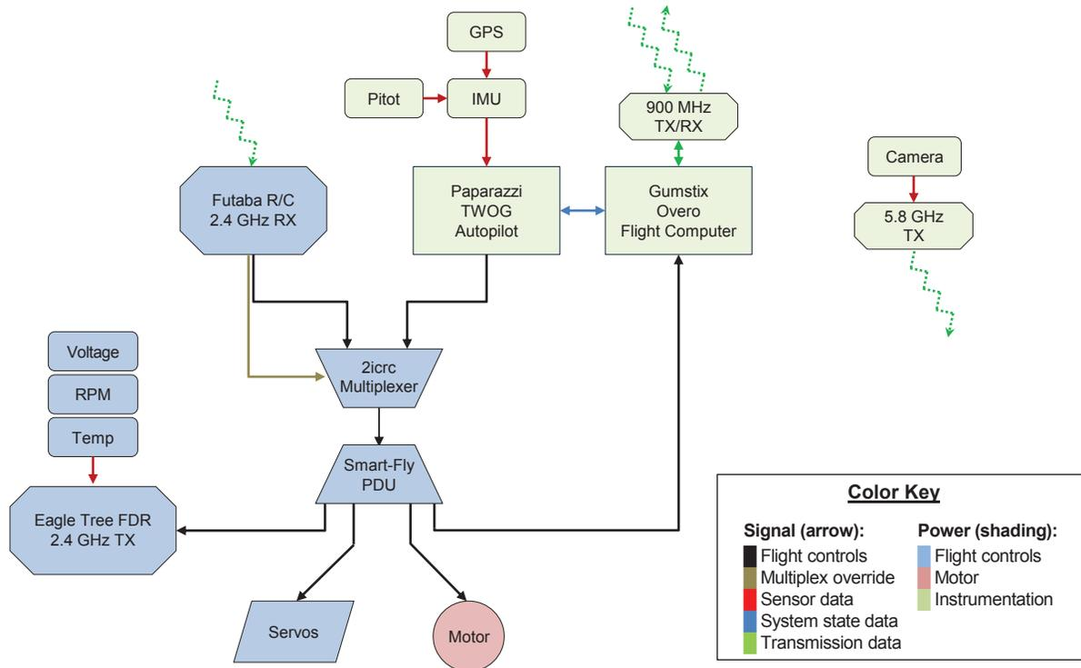
Figure 11. A flowchart diagram of the avionics suite showing a top-down view of flight control signals, multiplex the override command signal, sensor inputs, instrumentation communication, and transmission routes.
